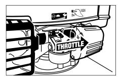
**Step 5** Slide the throttle control to the fast position.
